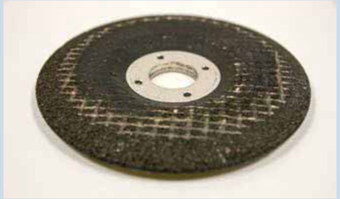
Defective grinding disc (the angle of attack is too flat)
